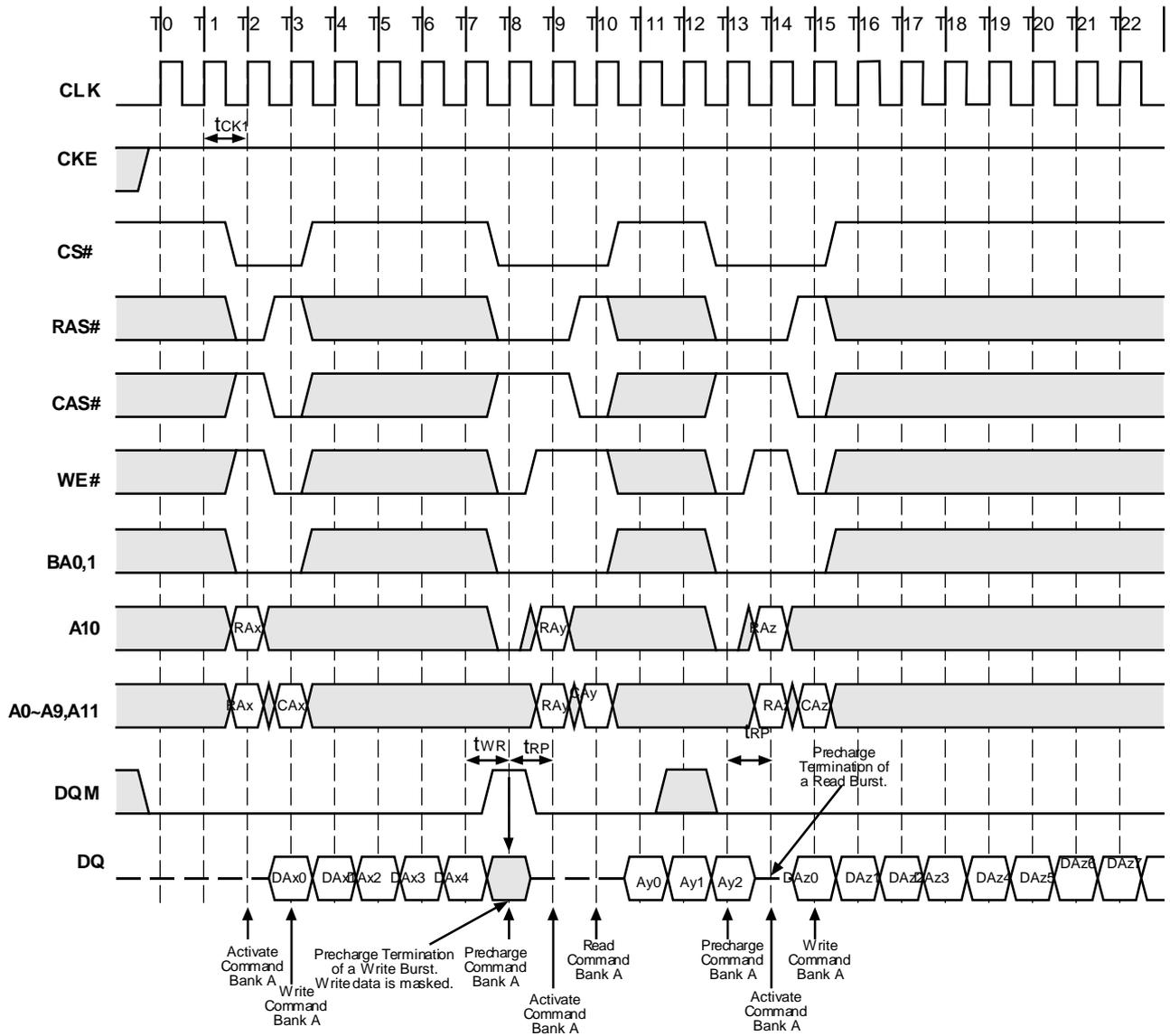
**Figure 24.2. Precharge Termination of a Burst**
