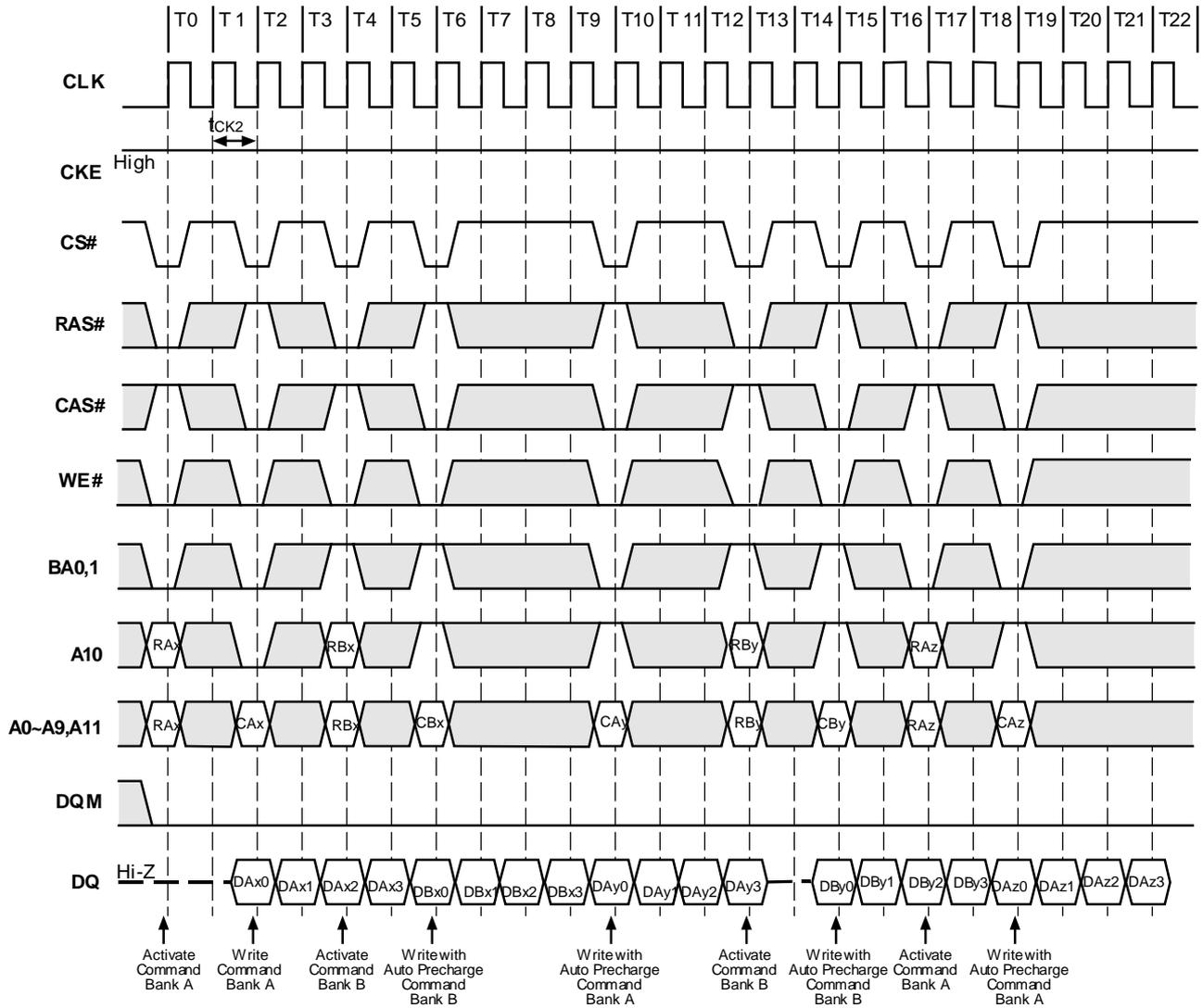
**Figure 17.3. Auto Precharge after Write Burst (Burst Length=4, CAS# Latency=3)**
