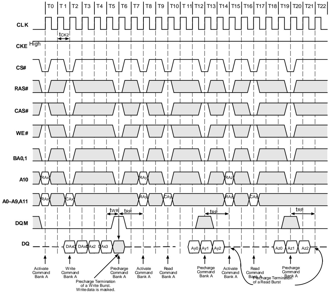
**Figure 24.3. Precharge Termination of a Burst**
