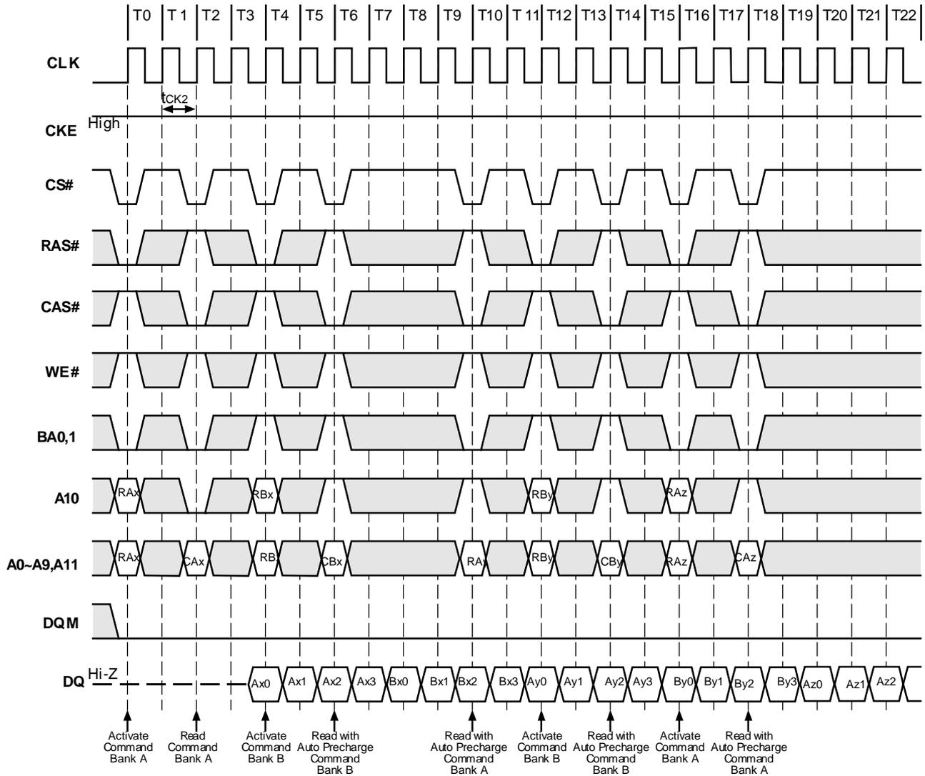
**Figure 16.3. Auto Precharge after Read Burst (Burst Length=4, CAS# Latency=3)**
