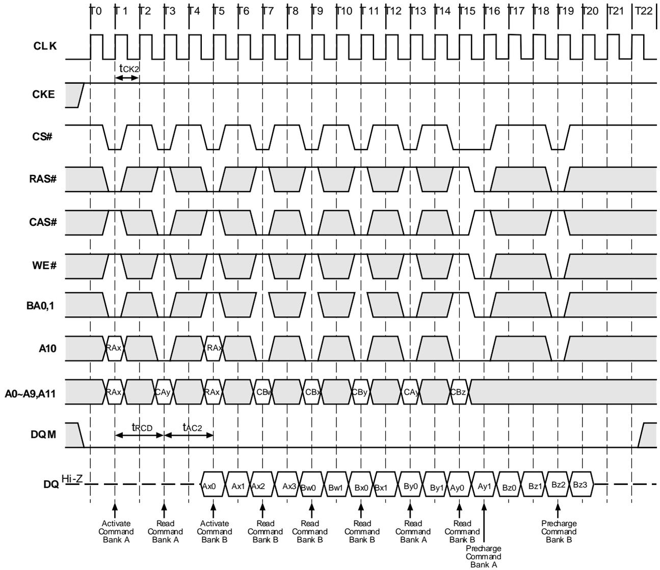
**Figure 14.3. Interleaved Column Read Cycle (Burst Length=4, CAS# Latency=3)**
