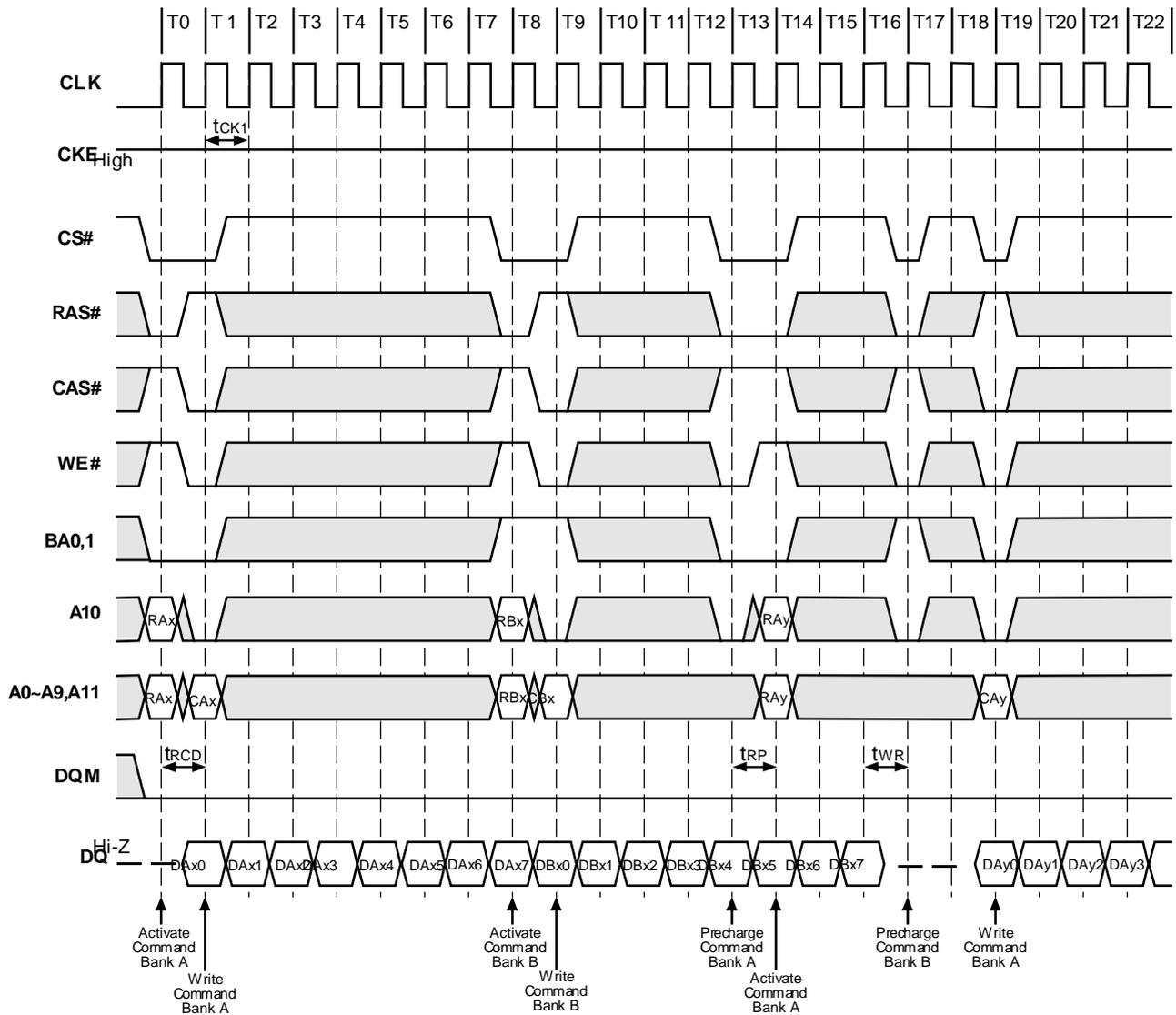
**Figure 12.2. Random Row Write (Interleaving Banks)**
