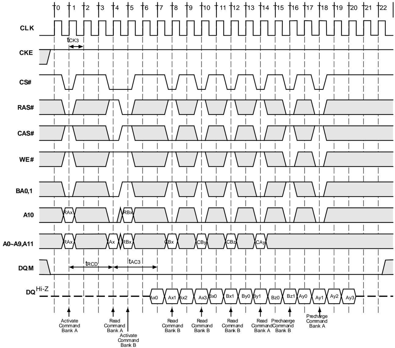
**Figure 15.1. Interleaved Column Write Cycle (Burst Length=4, CAS# Latency=1)**
