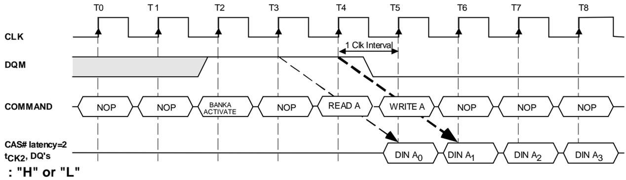
**Read to Write Interval (Burst Length <sup>3</sup> 4, CAS# Latency = 2)**
