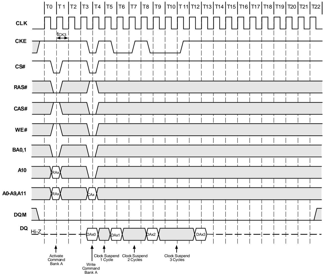
**Figure 8. Power Down Mode and Clock Mask (Burst Length=4, CAS# Latency=2)**
