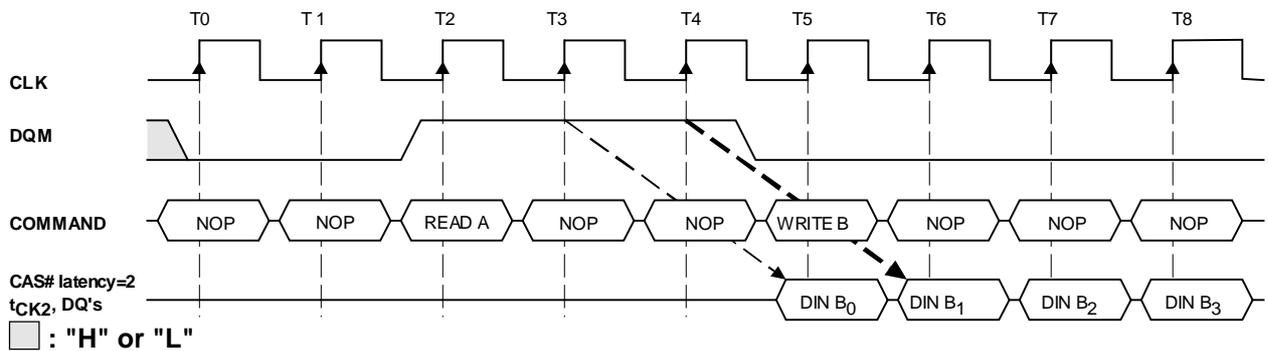
**Read to Write Interval (Burst Length <sup>3</sup> 4, CAS# Latency = 2)**
