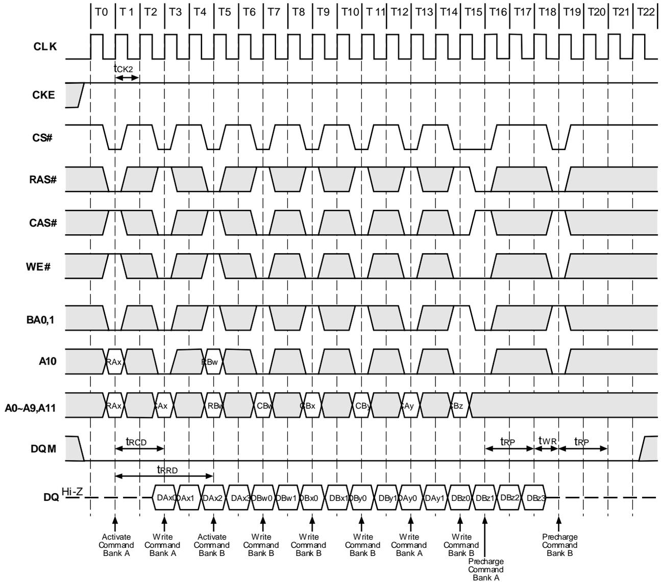
**Figure 15.3. Interleaved Column Write Cycle (Burst Length=4, CAS# Latency=3)**
