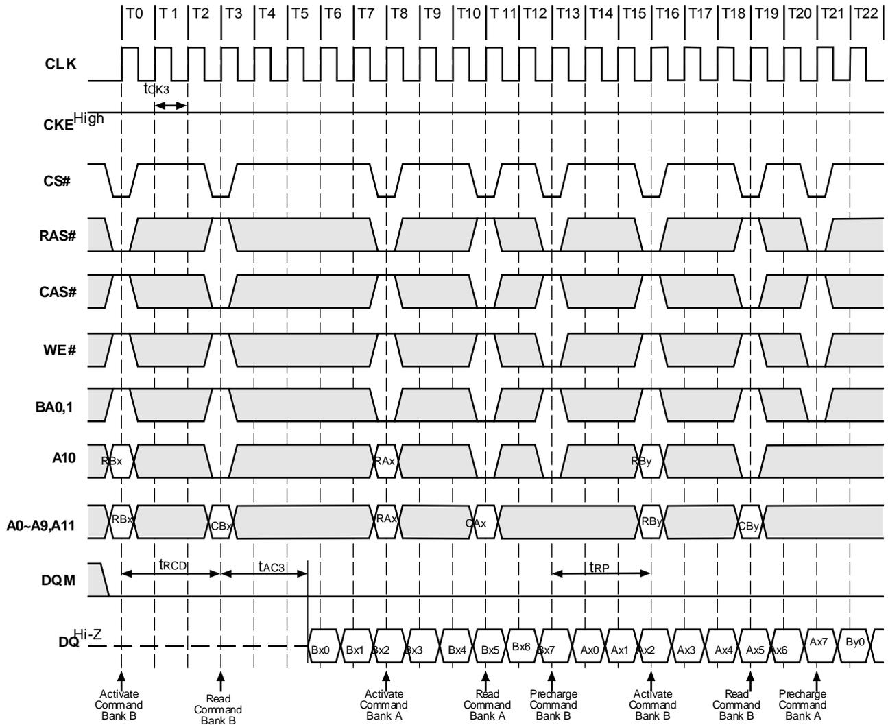
**Figure 12.1. Random Row Write (Interleaving Banks)**
