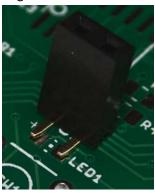
2. You will need to cut the LED leads so you can place the 3mm LED on the pin header so the case will just fit over the LED (remember to note the positive side of the LED). You will need to replace the standard 5mm buttons with the 20mm long buttons.
