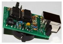
You can adjust this by cutting a small piece of the foam that came with the ATtiny85 and gluing it underneath the USB receptacle.
