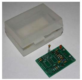
You can also choose to solder the thermistor with the leads intact so you can place the PCB in a small container and the thermistor's top would be located outside the container. You can also solder wires to position the thermistor elsewhere.
