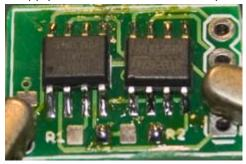
6. Position and hold the 10K thermistor (R1) in place using tweezers and solder the pin you previously applied a bit of solder to, and then apply solder to the other pin. Compared to the capacitor, the thermistor is slightly bigger.
