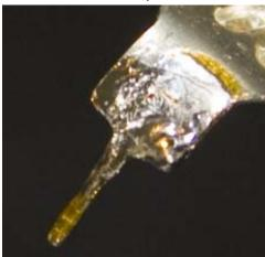
12. Install the battery holder pin and solder both sides. You can use sticky tape to hold it in place.
