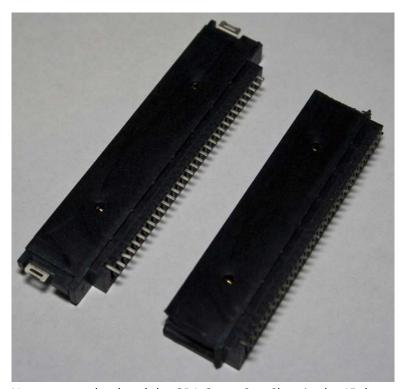
Next you need to bend the GBA Game Cart Slot pins by 45 degrees or thereabouts otherwise the pins will sit a few millimetres above the board. The GBA Game Cart Slot may also have two small little plastic bits on the bottom which you will need to shave off.
