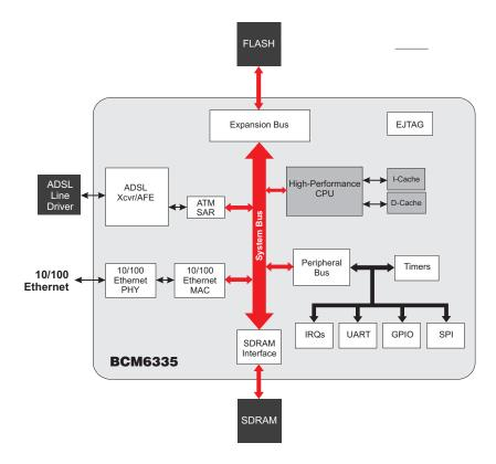
The **BCM6335** is a single-chip G.992.1/G.992.2/G.992.3 and T1.413 ADSL-to-Ethernet CPE router with a high-performance MIPS32<sup>TM</sup> CPU, a 10/100-Mbps Ethernet interface with Auto-MDIX, and FLASH and SDRAM interfaces.
