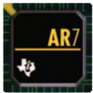
The AR7Wi chipset is a highly-integrated solution which places all of the needed wireless local area network (WLAN) components on the residential gateway's (RG) motherboard in
