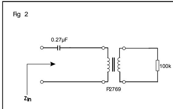
In practice, the  $100k\Omega$  load can be increased without limit. The DC blocking capacitor should be a minimum of  $0.22\mu F$  to avoid resonance within the voiceband to obtain a flat frequency response and input impedance to specification.
