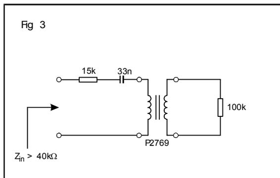
At the expense of a small loss, (approximately 1.5dBV) the circuit in fig.3 provides an impedance exceeding  $40k\Omega$ , 200Hz – 4.3kHz, and frequency response flatness within  $\pm 0.25dB$  over the same band.
