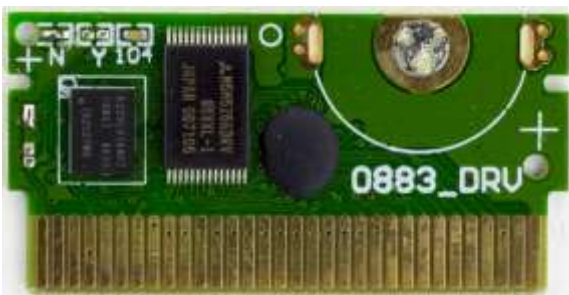
ES29LV160 Flash (0883_DRV PCB) - 1MByte Flash Cart (Requires 3.3V to erase/program)
