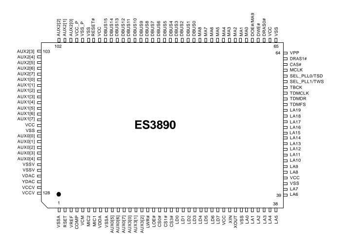
Figure 1 ES3890 Device Pinout
