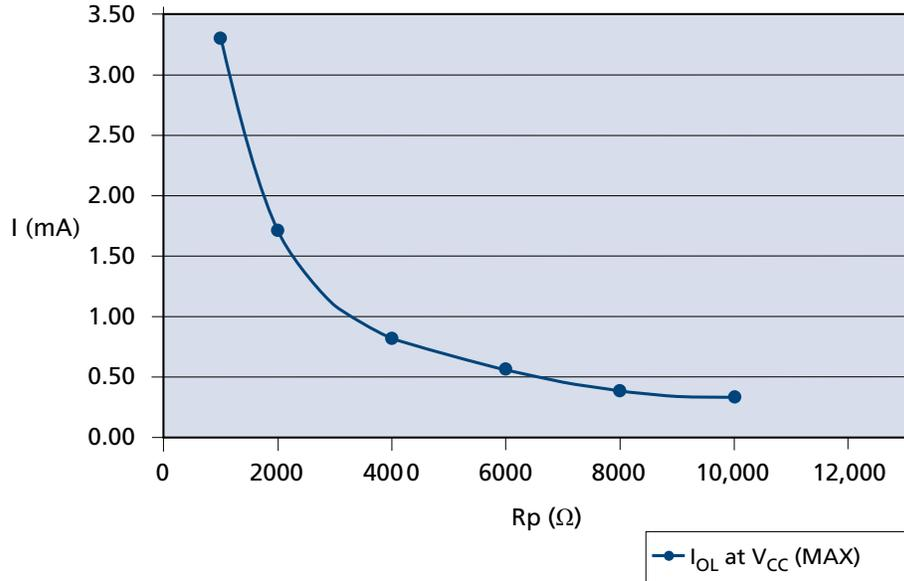
**Figure 20:  $I_{OL}$  vs.  $R_p$  (1.8V  $V_{CC}$ )**
